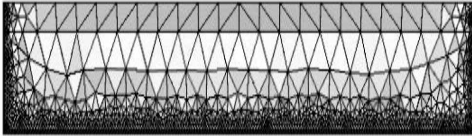
Figure 3. Meshing of a cylindrical 18650 cell.
