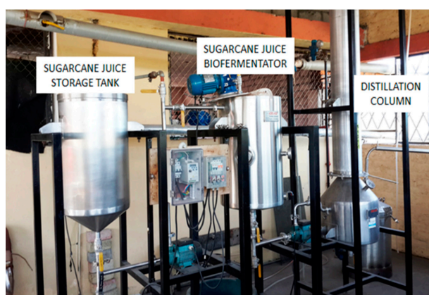
Figure 2. Fermentation of cane juice for bioethanol production in the pilot plant.
