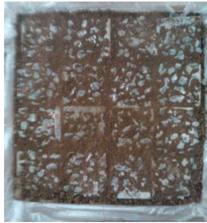
Figure 6. Vegetation-pervious concrete filled with mulching materials.
