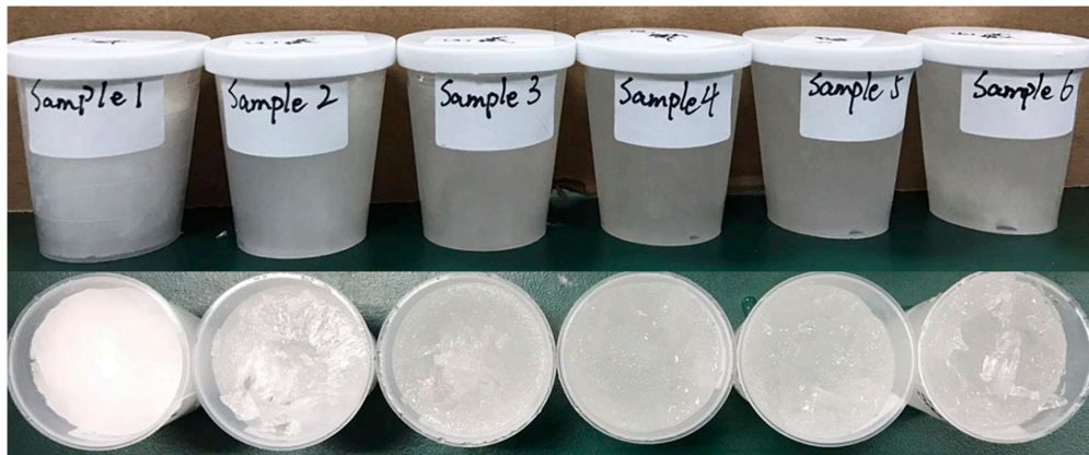
Figure 3. The photo of the prepared six samples containing different volumes of \text{CaCl}_2 \cdot 2\text{H}_2\text{O} and \text{CaCl}_2 .
