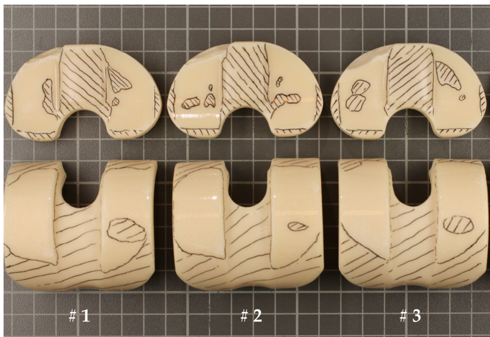
Figure 4. Worn areas on the three (#1–#3) tested BS-cement specimens.
