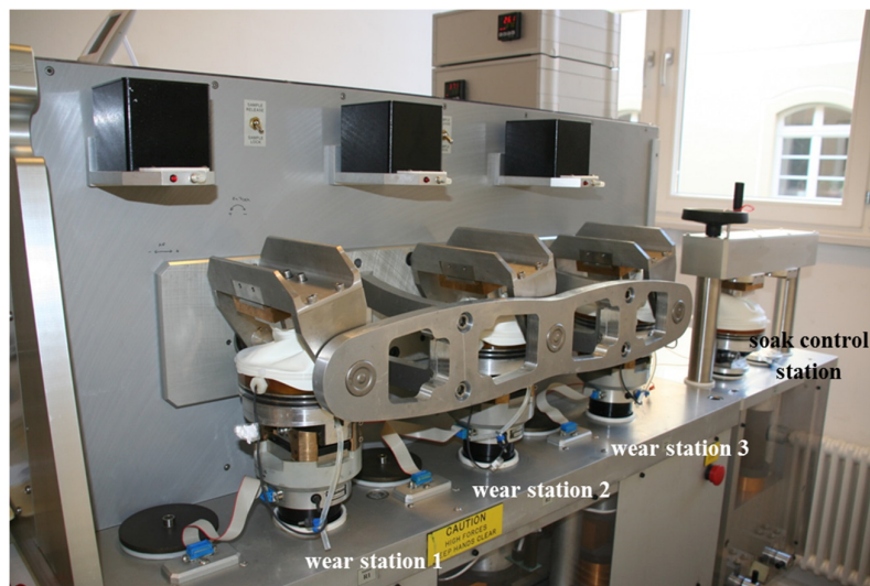
Figure 2. Knee wear simulator with three wear stations and one soak control station.
