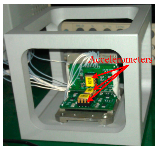
Figure 6. Mounted accelerometers in the test.
