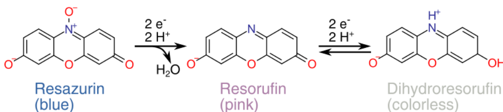
Scheme S1. (a) Photoreduction of resazurin to resorufin and further to dihydroresorufin associated with the color changes.
