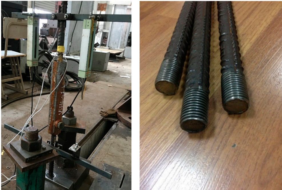
Figure 2. Test setup for specimens under incremental tensile load.
