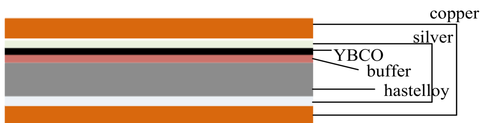
Figure 1. Typical configuration of 2G HTS tape.
