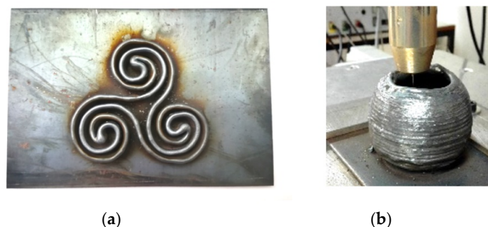
Figure 2. Examples of geometries obtained by WAAM: (a) Piece obtained by continuous trajectory and complex geometry in x-y direction; (b) Piece obtained by continuous trajectory and growing geometry in z direction.
