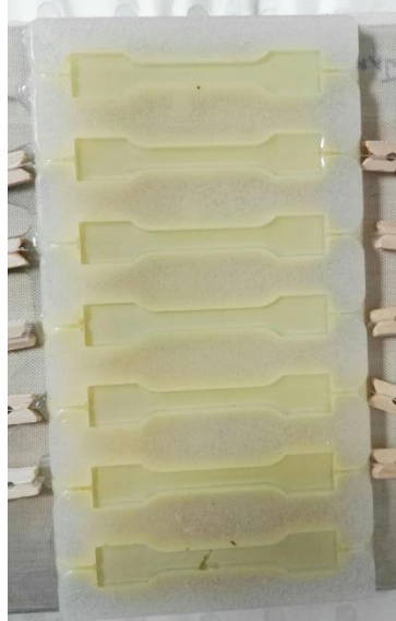
Figure S2 (ESI). Silicon SFFT mould with clear resin and fibers tensioned across the center.
