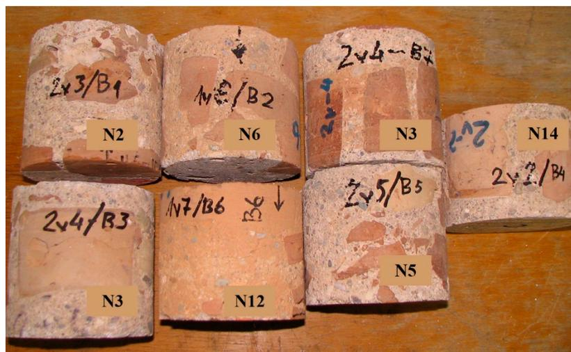
**Figure 5.** Specimens for compressive strength testing.
