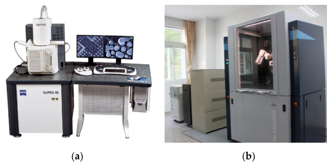
Figure 4. The test instruments: (a) the Zeiss Supra 55 field emission scanning electron microscope; (b) the D8-Advance type crystal X-ray diffractometer.
