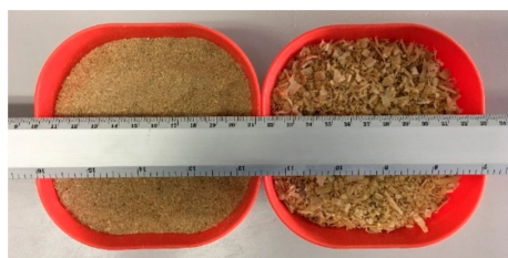
Figure 1. Sawdust and wood shavings used as raw material in the development of the new gypsum plasters.
