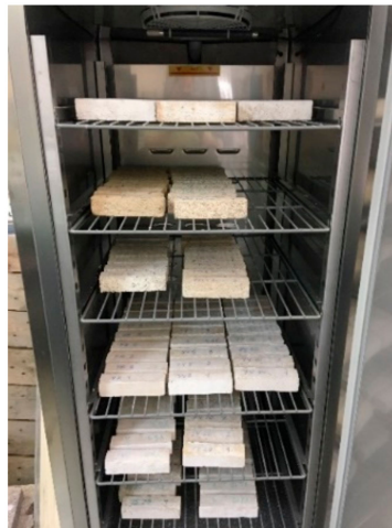
Figure 4. Samples during the wetting–drying cycles in the curing chamber.
