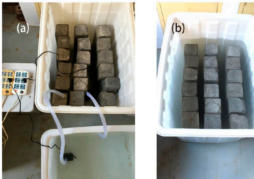
Figure 2. Curing methods of specimens; (a) schematic of the setup of the wet/dry cycles, (b) schematic of the setup of the immersion.
