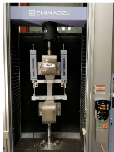
Figure 1. Direct tensile test setup.
