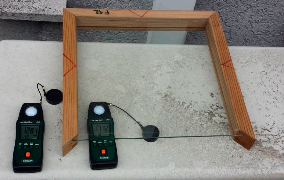
Figure S2. Measurements of light transmittance by means of Lux meter.
