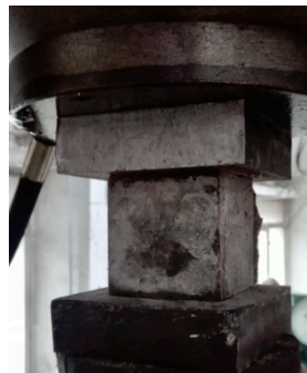
Figure 2. The cubic specimen subjected the compression test.
