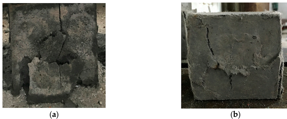
Figure 7. Examples of failed engineered cementitious composite (ECC) compression test specimens with different polyvinyl alcohol (PVA) fiber reinforcement conditions: (a) without fiber; (b) 1.0 vol.% PVA fiber.
