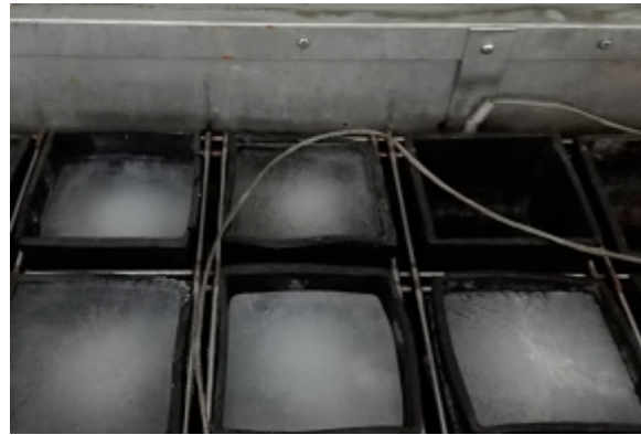
Figure 5. Freeze–thaw test specimens placed in the chamber.
