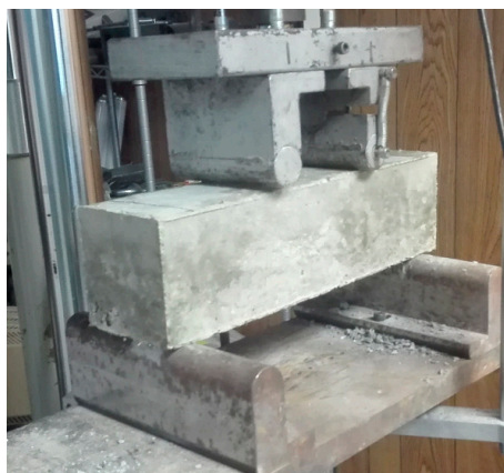
Figure 3. The prismatic specimen subjected to the flexure test.
