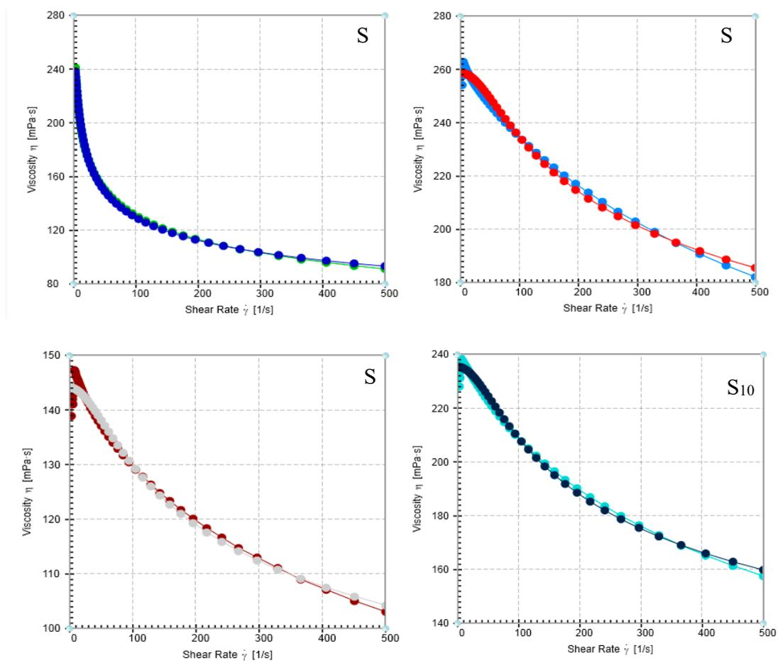
**Figure S5.** Representative plots of viscosity (vs.) shear rate for selected formulations S1 (1:1:1); S2 (3:0:0); S6(0:0:3) and S10(0:3:0).
