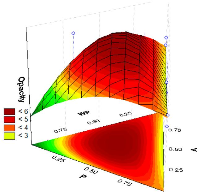
**Figure S2.** 3D surface plot of the effects of components on opacity of edible films where the interaction of WP with P/A increased the opaqueness.
