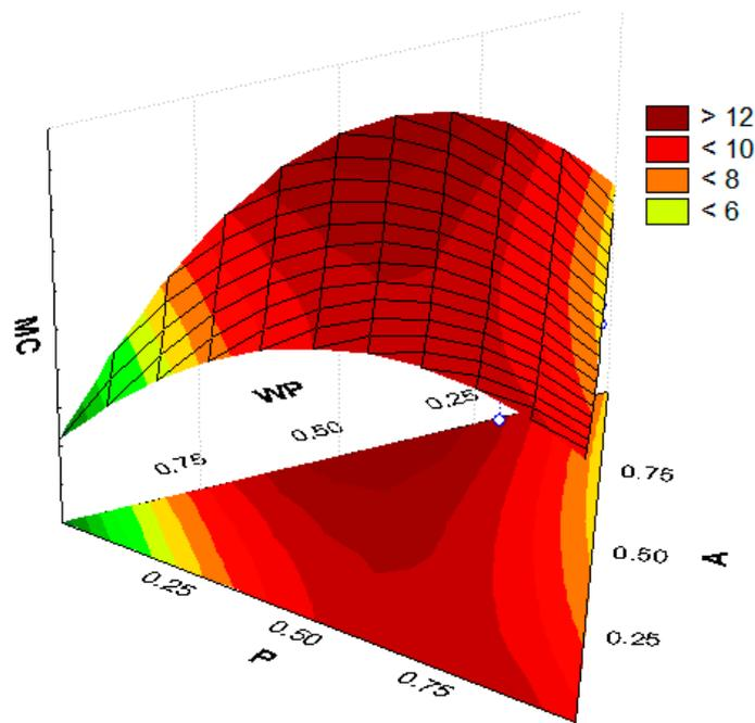
**Figure S3.** 3D surface plot of the effects of components on Moisture content (%) of edible films.
