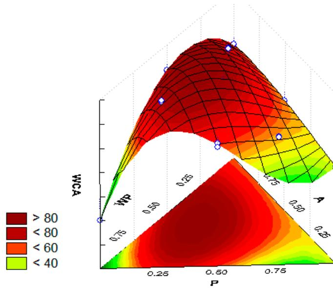
**Figure S4.** 3D surface plot of the effects of components on water contact angle ( $\theta$ ) of edible films where the blending of WP/P/A results in higher convexity indicating improved hydrophobicity of films.
