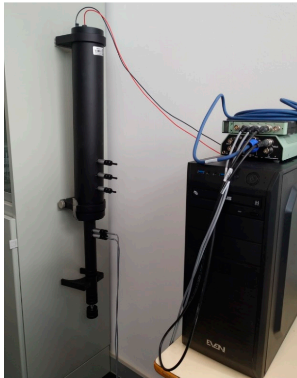
Figure 1. Impedance tube: experimental setup.
