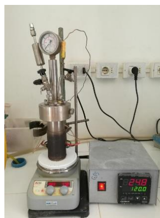
Scheme S1. Semi-Batch reactor used for the catalytic measurements.
