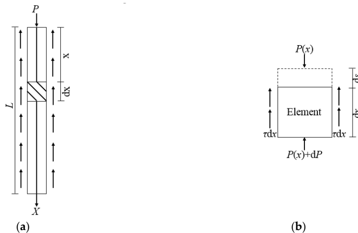
Figure 9. Diagram of force analysis of I-shaped steel. (a) Force diagram of detached body; (b) Force diagram of element body.
