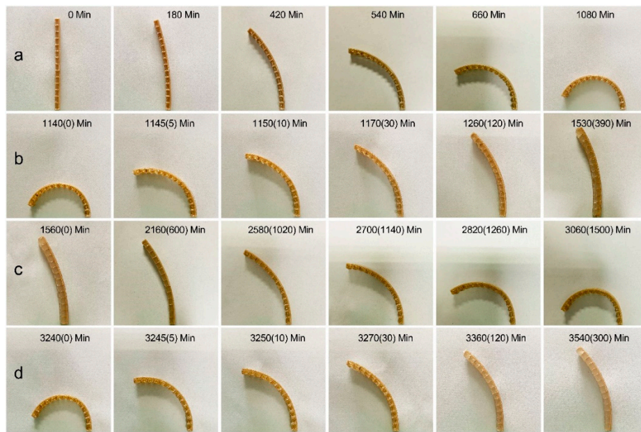
Figure 3. The bio-hygromorph self-shaping during the desorption-absorption cycle: (a) bending during the desorption stage of the first cycle; (b) straightening during the absorption stage of the first cycle; (c,d) are deformations during the desorption and the absorption stages of the second cycle, respectively.
