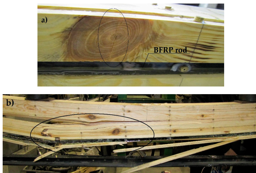
Figure 14. Image of the Wa-B2 beam's destruction: (a) cracking of a deteriorating oval knot, (b) cracking of burls near knots and spiral grains (photograph by Wdowiak).
