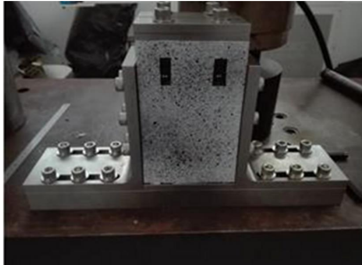
Figure 4. Edge-constraint structure adopted in the experiment.
