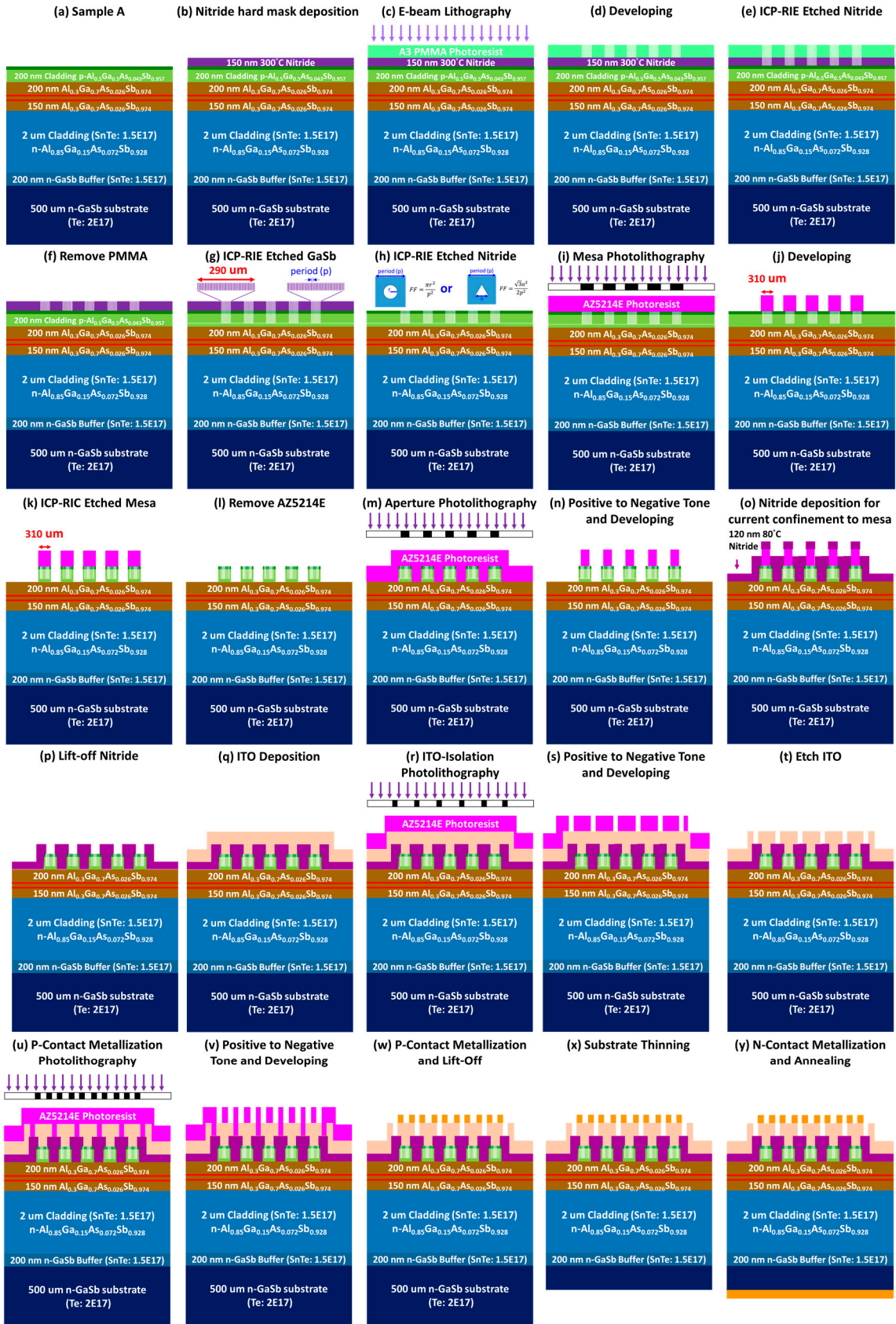
Figure S3. Fabrication process of electrically pumped PCSEL device based on sample A.
