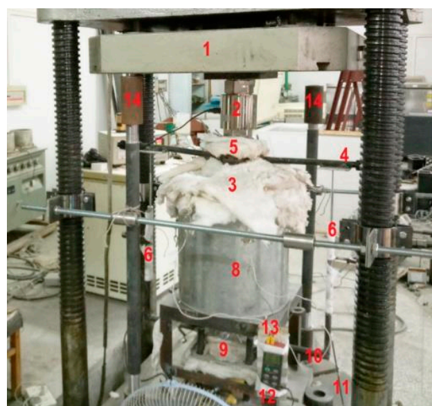
(a) Test-setup for simultaneous heating and loading
