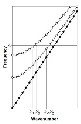
**Figure 2.** Schematic illustration of the band structure of the three coupled one-dimensional elastic waveguides.  $\omega$  is the frequency of the external driving force. The wavenumbers of the states with the largest amplitudes along the two bands with cut-off frequencies are labelled on the wavenumber axis.
