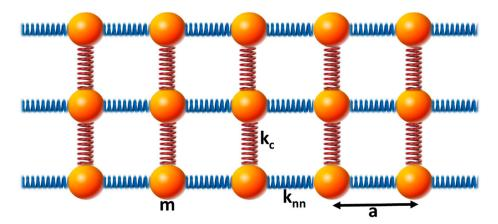
**Figure 1.** Schematic illustration of the system composed of three coupled one-dimensional elastic waveguides. The red springs couple the three elastic chains identified with blue springs. See text for meaning of symbols.
