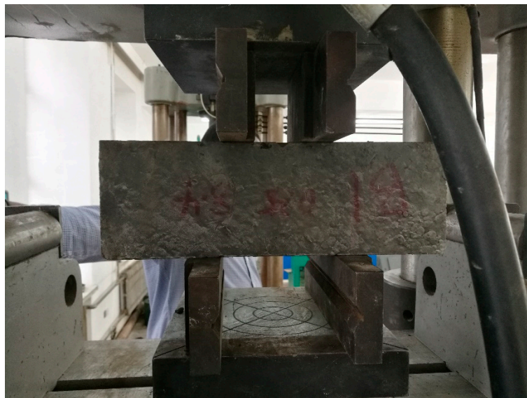
Figure 1. Direct shear test experimental set-up.
