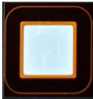
Figure 2. Optical microscopic image of the fabricated SiC PiN diode with an active area of 0.1 \text{ cm}^2 ( 0.28 \text{ cm}^2 chip size).
