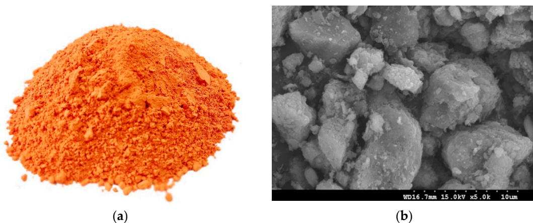
Figure 3. (a) Calcined Hwangtoh powder. (b) SEM micrographs of calcined Hwangtoh.
