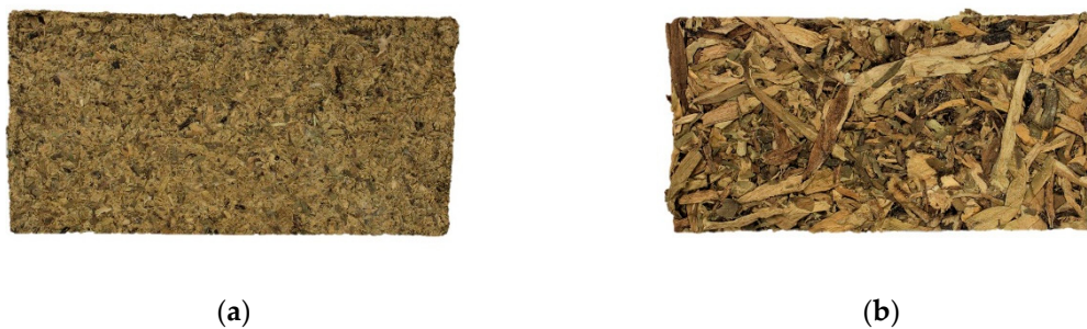
Figure 2. Manufactured Binder-Less WHP panels: (a) pulp WHP: Panel made with pulp (WHP passing through #2 sieve, R20); (b) staple WHP: Panel made with staple (WHP retained on #2 sieve, R20).
