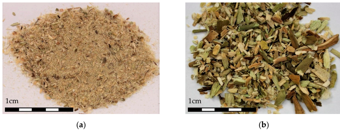
Figure 1. Final Water Hyacinth Petiole (WHP) appearance after the crushing process: pulp (a) and staple (b).
