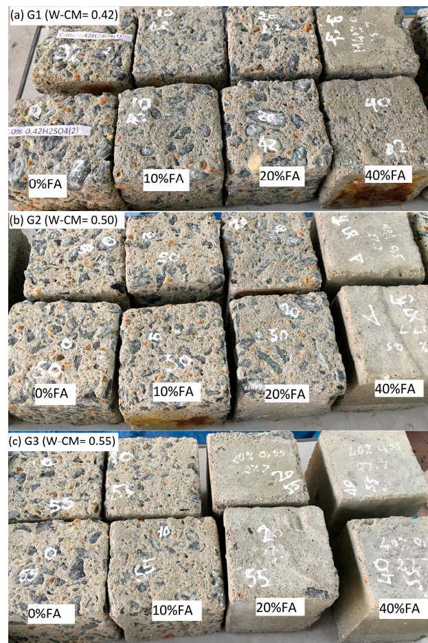
Figure 5. Surface appearance of concrete cubes after immersion in 10% sulfuric acid solution. (a) G1 (W–CM = 0.42); (b) G2 (W–CM = 0.50); (c) G3 (W–CM = 0.55).
