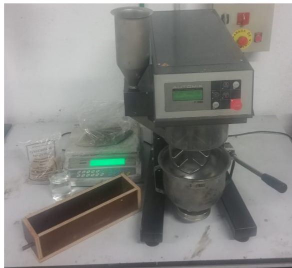
Figure 1. Photo of the wooden mold with the steel bar, the mortar mixer, and the materials used: cement (on top of the balance), siliceous sand, and water containing the proper amount of dissolved NaCl.
