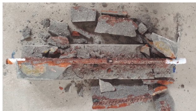
Figure 6. Photo taken after breaking the M1-reinforced mortar specimen at the end of the corrosion test.
