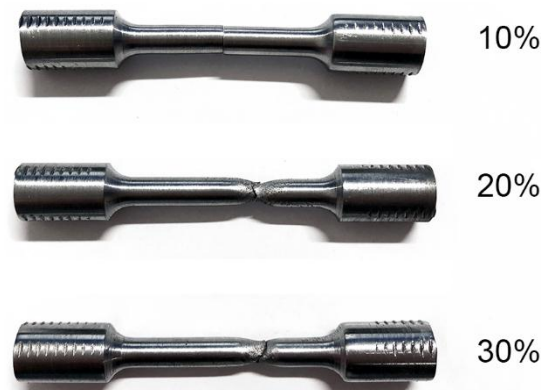
Figure 8. Room-temperature tensile macroscopic fractographs of the crack healing zones under different reduction ratios, healing at 950 °C for 10 h.
