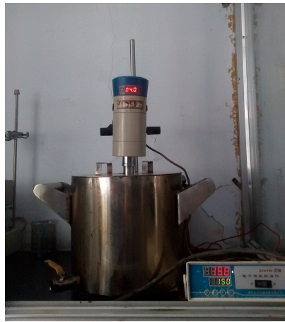
Figure 2. Mixing process of asphalt modification.
