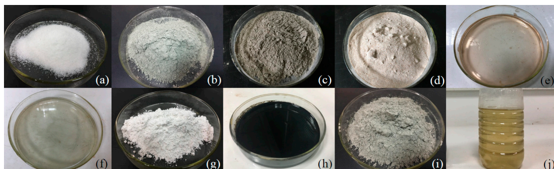
Figure 1. Cements and additives, (a) super absorbent polymer (SAP), (b) ordinary Portland cement (PO), (c) fly ash, (d) activator of the geopolymer, (e) anti-freezing agent (AFA), (f) early strength agent (ESA), (g) metakaolin (MK), (h) EN-1, (i) inorganic additive from Xi'an, (j) Toogood.
