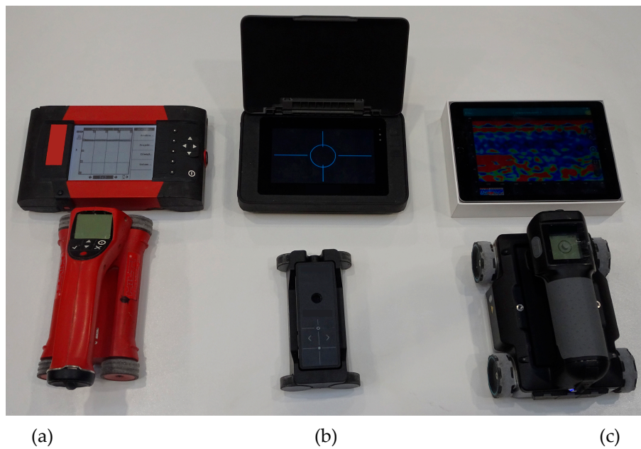
Figure 9. Devices used in tests, (a) electromagnetic device (1), (b) electromagnetic device (2), and (c) radar device (3).
