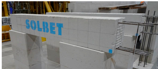
Figure 5. Tested elements with the reinforcement broken down at its ends.
