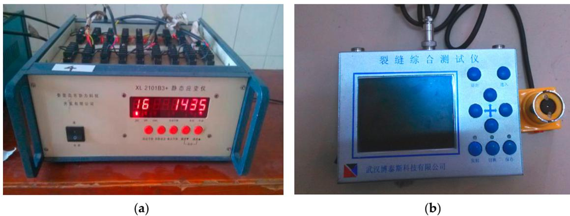
**Figure 8.** Instruments for the plat-ring-type test: (a) static strain testing device; (b) crack testing device.
