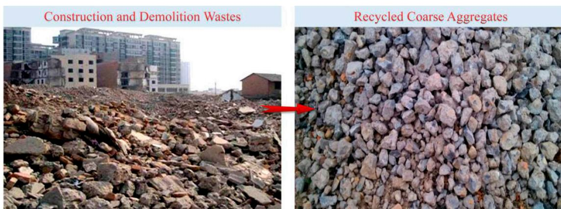
Figure 1. Recycled coarse aggregates.
