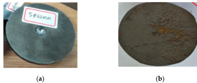
Figure 14. Comparable analysis of void closure in the core of specimen. (a) before floating pressure; (b) after floating pressure.
