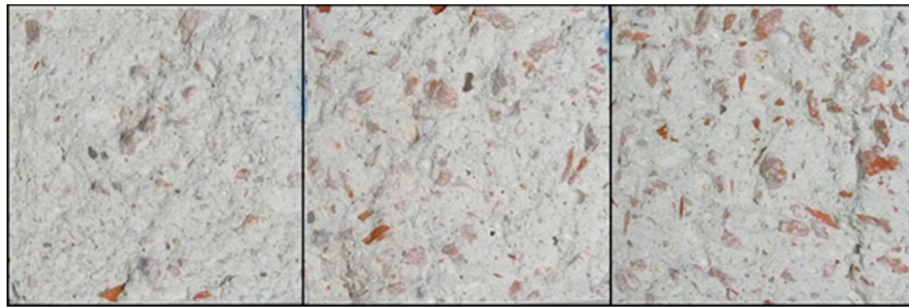
Figure 4. Compounds containing 25% ( left ), 50% ( center ), and 75% ( right ) of mixed waste (concrete and ceramic).
