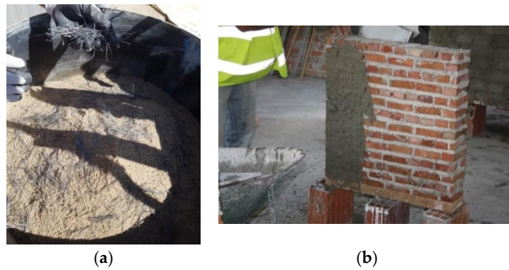
Figure 11. Reinforcement preparation: (a) mixing polypropylene fibers with sand and (b) application.
