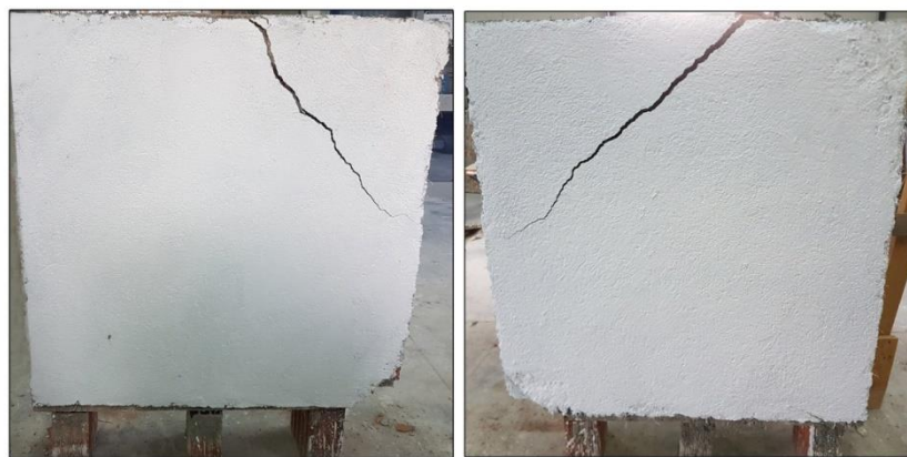
Figure 17. Failure mode of W-6-PF.
