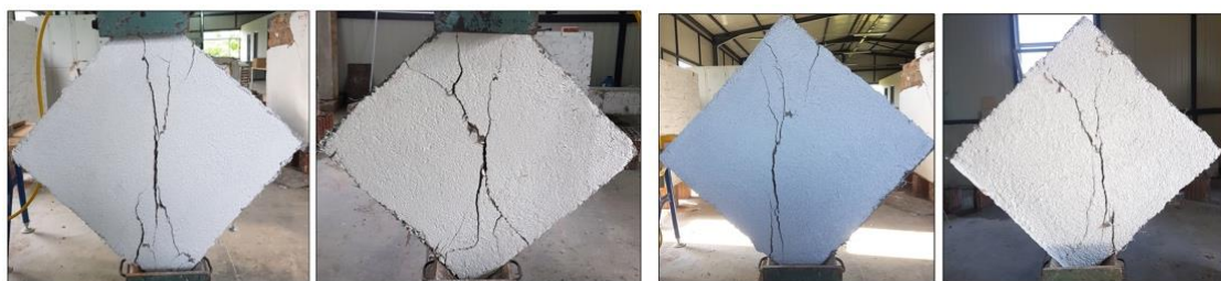
Figure 18. Failure mode of SW-3-PF.
