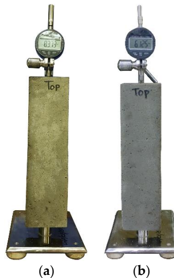
Figure 3. Measurement of concrete expansion made with 100% BA (a) and 100% SSA (b).
