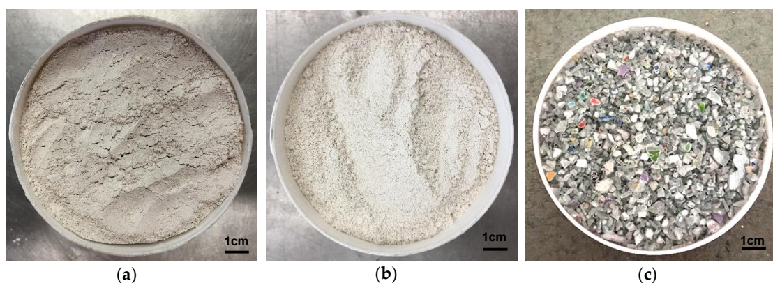
Figure 1. Materials used to develop the new plasters: (a) commercial gypsum; (b) unheated gypsum waste from plasterboard production; (c) polycarbonate waste.
