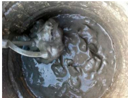
Figure 2. Cement paste mixed basalt fiber directly.
