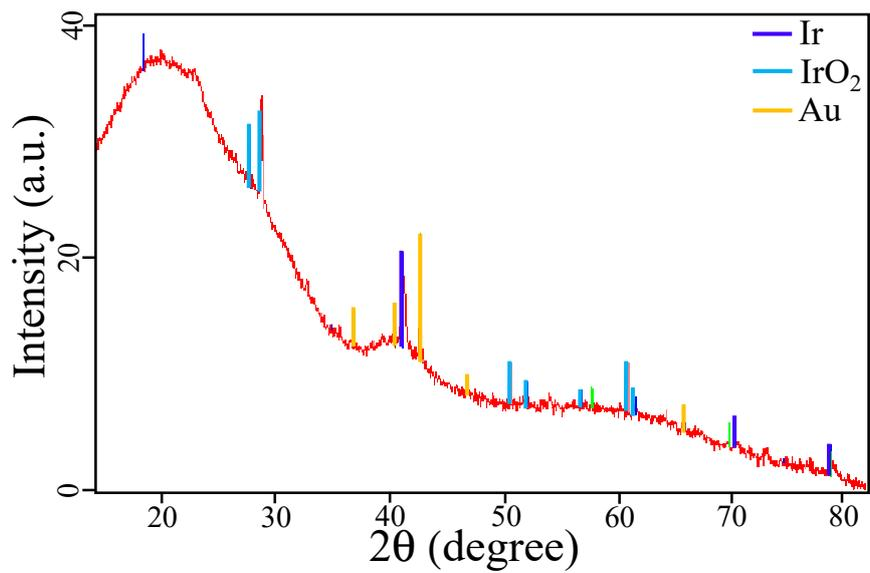
**Figure S7.** XRD pattern of iridium-gold (Ir-Au) microstructures.
