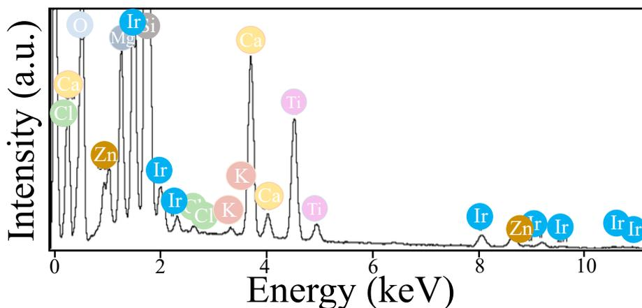
Figure S2. EDX spectrum of iridium (Ir) microstructures.
