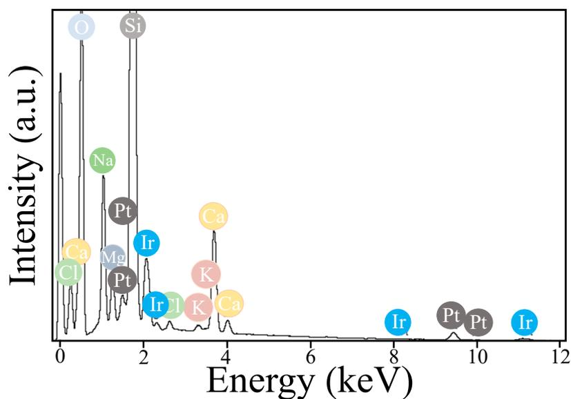
Figure S3. EDX spectrum of iridium-platinum (Ir-Pt) microstructures.
