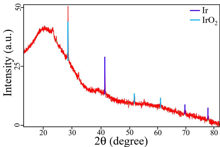
**Figure S5.** XRD pattern of iridium (Ir) microstructures.
