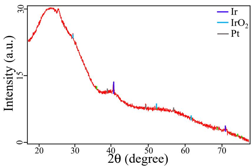
**Figure S6.** XRD pattern of iridium-platinum (Ir-Pt) microstructures.
