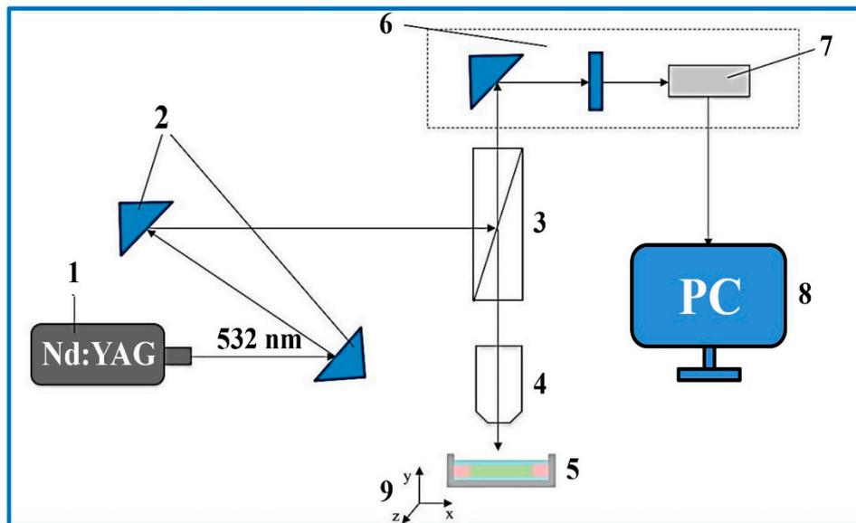
**Figure S1.** The experimental setup used for laser-induced deposition of iridium-containing microstructures: 1—cw 532 nm diode-pumped solid-state Nd:YAG laser, 2—mirrors, 3—splitting cube, 4—objective lens, 5—the experimental cell, 6—neutral density filter, 7—web camera, .
