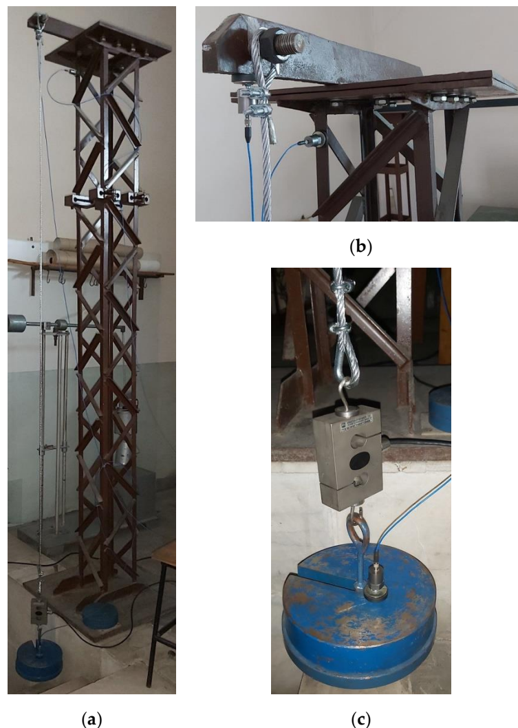
Figure 1. The experimental setup: (a) full view of laboratory stand; (b) detail view of rigid tower upper side device for hanging the wire rope, with parasite motions monitoring transducers; and (c) detailed view of loading mass ensemble, with force and acceleration transducers.
