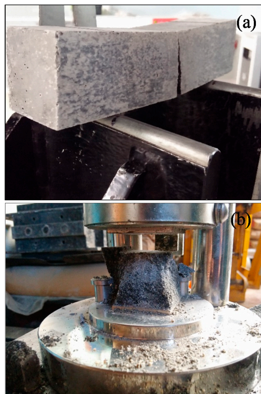
Figure 10. Images of specimens after tests: (a) specimen GC (0.5%) after flexural test, (b) specimen GC (0.5%) after compression test.
