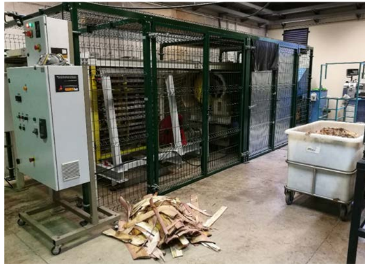
Figure 1. Pilot plant for extraction of banana fiber.
