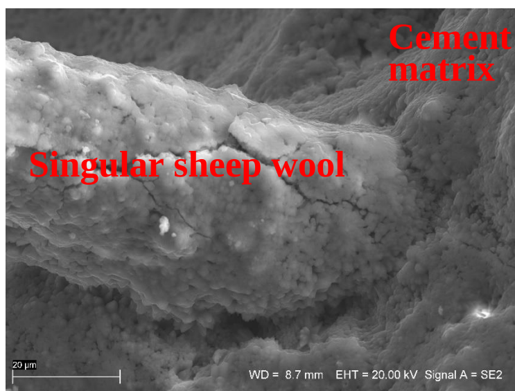
Figure 7. SE image of the sheep wool fibre—interface—cement matrix, scale bar = 20 µm.
